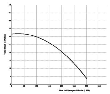
Note: Performance based on pumping solvent (0.78 specific gravity). Pressure is taken at the manifold discharge outlet. Fixed Speed 1.5 HP was powered by Single-Phase, 50 Hz, 250 Volt incoming supply. (STP150C)
