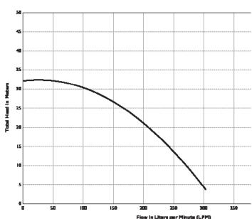
Note: Performance based on pumping solvent (0.78 specific gravity). Pressure is taken at the manifold discharge outlet. Fixed Speed 1.50 HP was powered by Three-Phase, 50 Hz, 415 Volt incoming supply.
